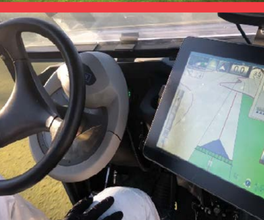
GPS sprayer application on a fairway. Auto-steer is guiding the sprayer and application coverage is being displayed on the GPS screen.
